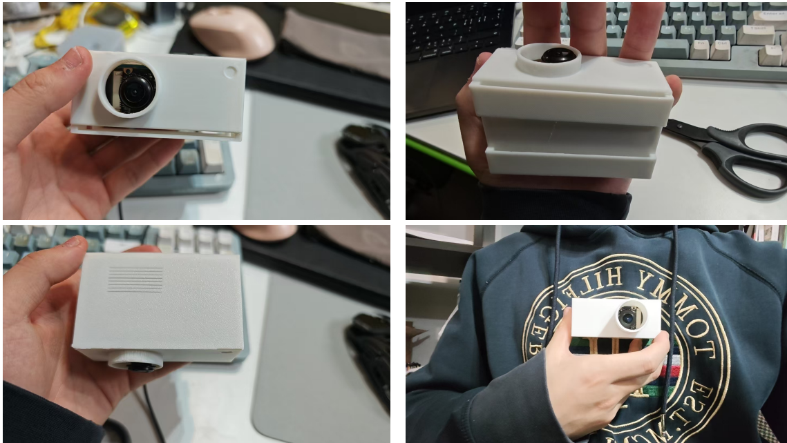
Fig. 6. Hardware prototype of Touvigation shown from the front, side, top, and worn views. The prototype combines a head-mounted egocentric camera, a custom 3D-printed support structure, onboard Raspberry Pi computing, speech input, and audio output into a single wearable system.
